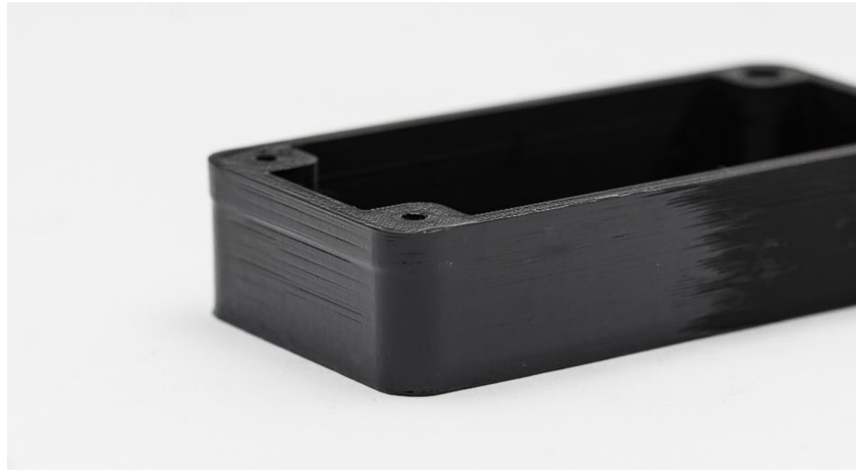
A black print showing half coated with epoxy and half unprocessed
