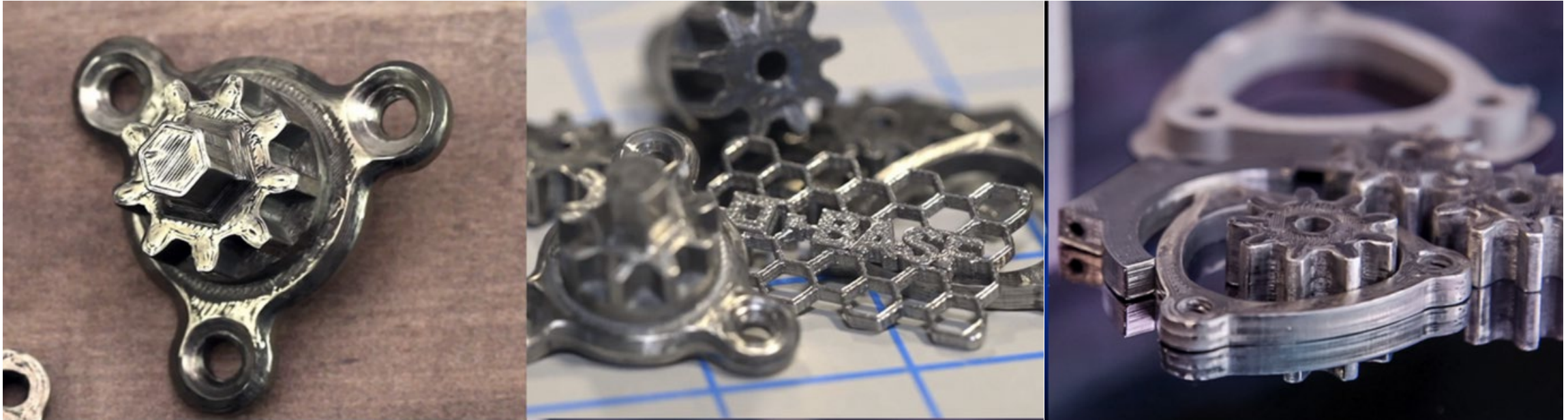
Metal Filled Filament MEX Printed Sample Parts
