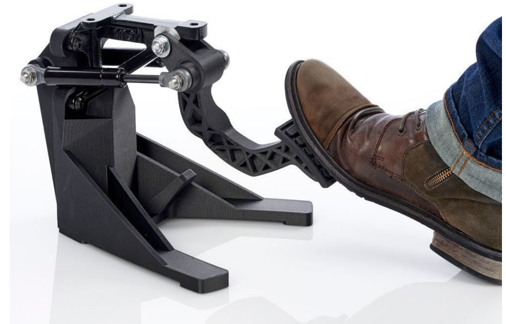
AM Printed Brake Pedal Assembly
