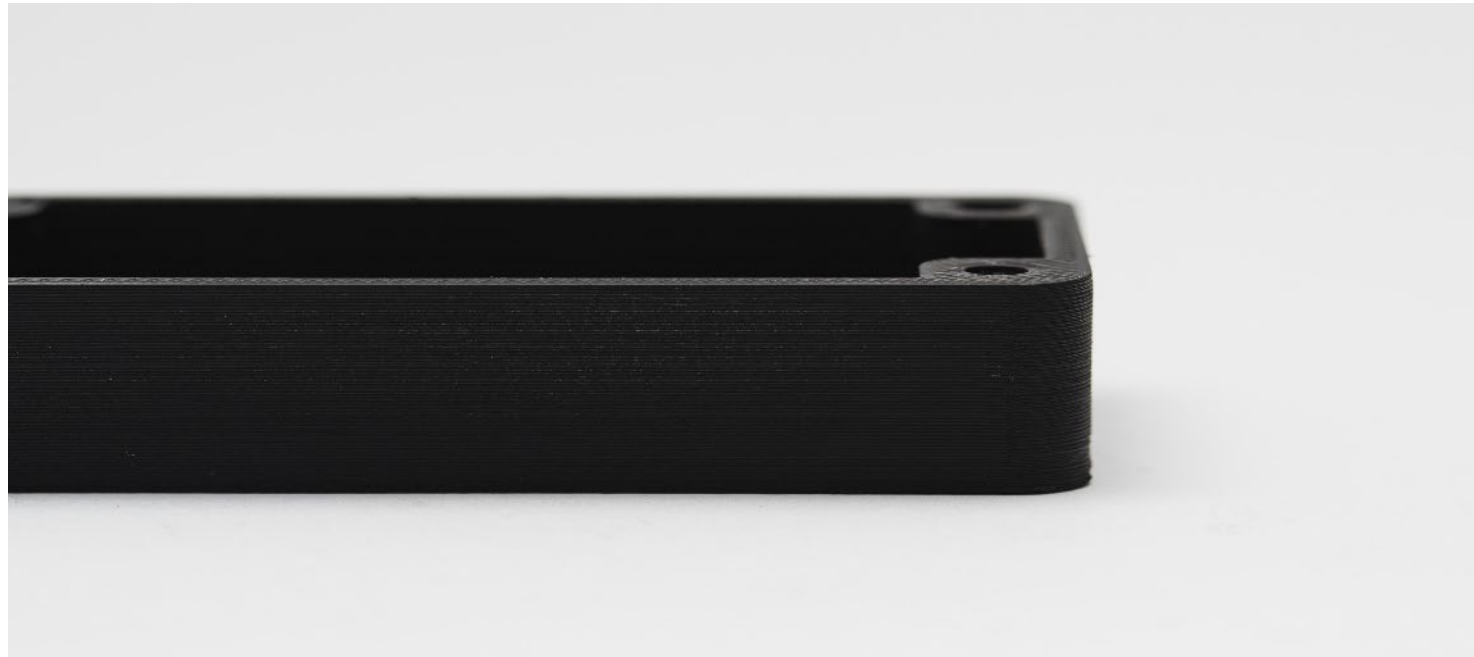
A grey PLA Material Extrusion print spray painted black
