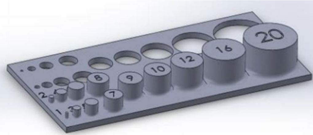
Holes & bosses (horizontal/vertical) test
