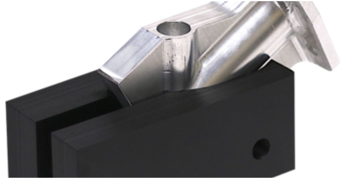
Fiberglass filled AM Printed Soft Jaws
