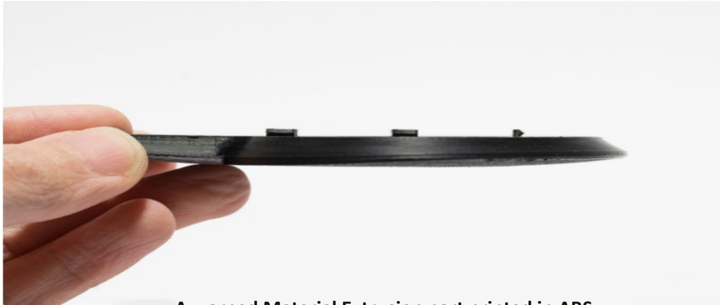
A warped Material Extrusion part printed in ABS
