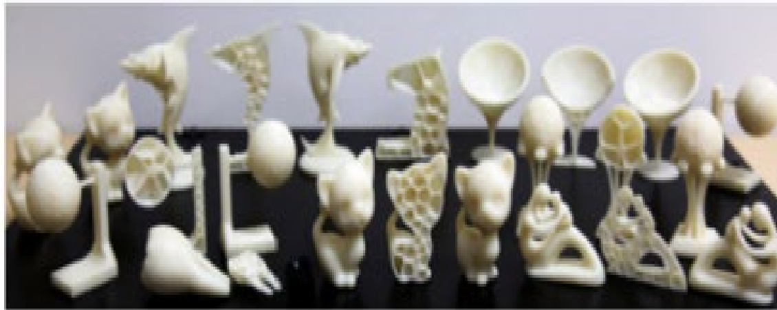
Honeycomb Support - Material Extrusion
