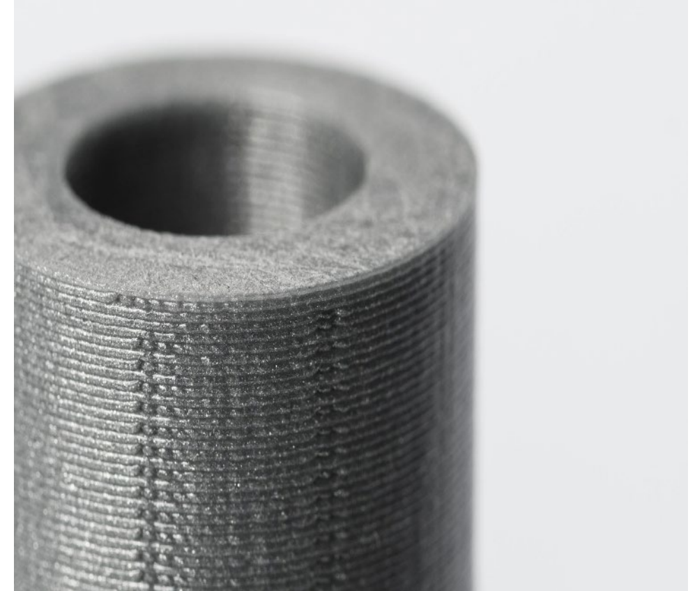
The layer lines of an Material Extrusion part are generally visible
